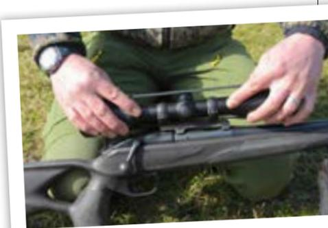
Place the rings as far apart as possible for stability and to distribute the weight of the scope
